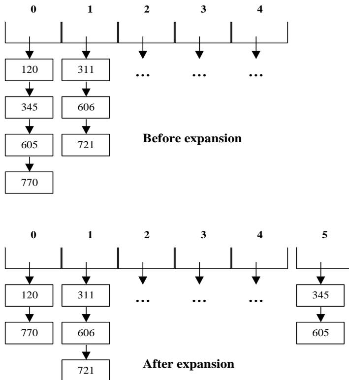
**Figure 2: Splitting bucket 0 in a five-bucket table.**
