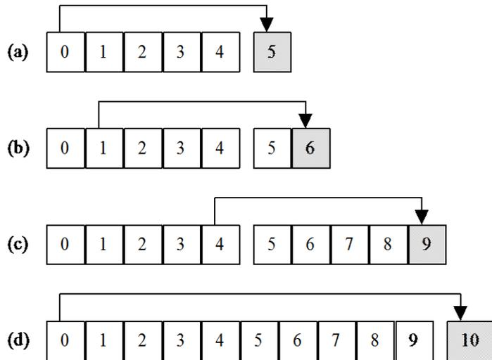
**Figure 1: Expansion process of linear hashing for a five-bucket table**
